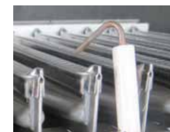
Electrode assembled on the manifold side
